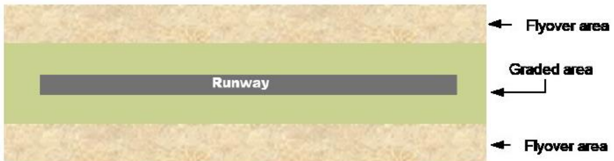
Figure 1: Composition of a runway strip
