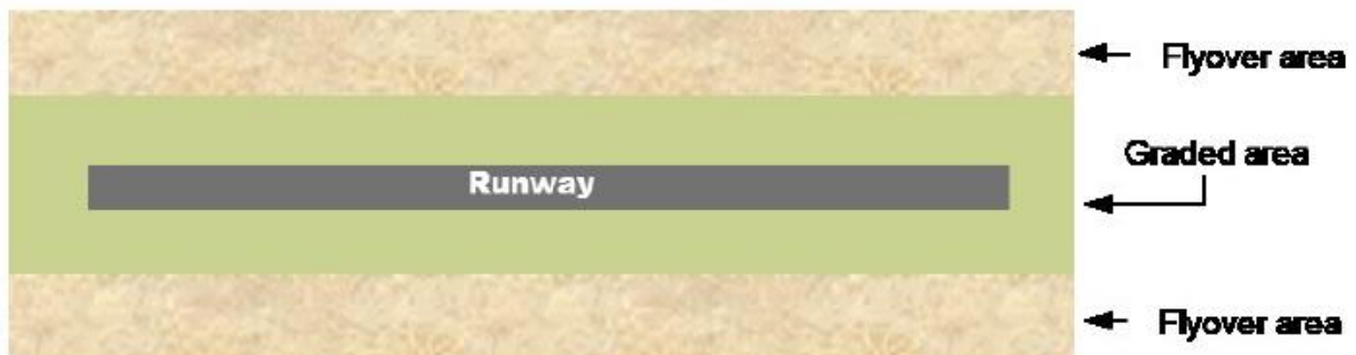
Figure 1: Composition of a runway strip
