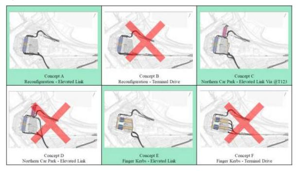
A preferred option was identified involving repurposing level 3 with 'finger' kerbs for pick-up/drop-off (Concept 'E' in the preceding figure). This layout uses side-to-kerb configuration for vehicles to drop-off and pick-up, set-out in parallel rows to enable maximum throughput capacity, and ensures vehicles do not need to reverse which provides safety benefits. Dual sided finger kerbs are used in other major international airports, including London Heathrow Airport.
