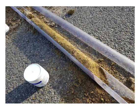
Photo 3. Orange-brown sandy clay material encountered beneath silty clay at some locations.
