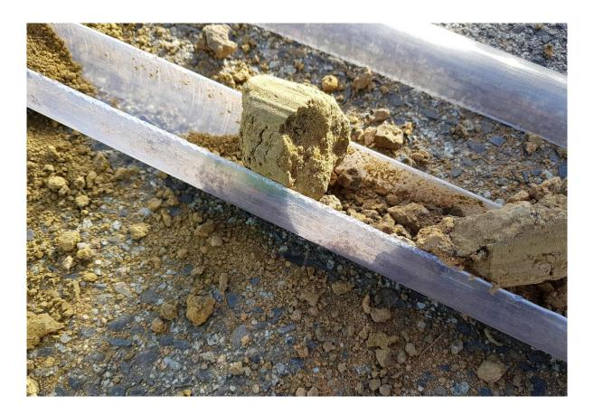
Photo 5. Orange-brown clayey sand with basalt gravels encountered within some locations.
