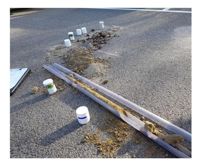
Photo 2. Lithology encountered ranging from gravelly fill to silty clay, becoming sandy with weathered basalt gravels with increasing depth.
