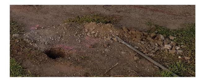
Photo 1. Lithology encountered ranging shallow gravelly fill (left) to silty clay with calcareous inclusions (right).
