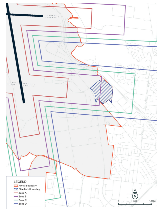
Figure 8.17 Melbourne Airport light control zones interaction with Elite Park (ultimate four-runway configuration)
