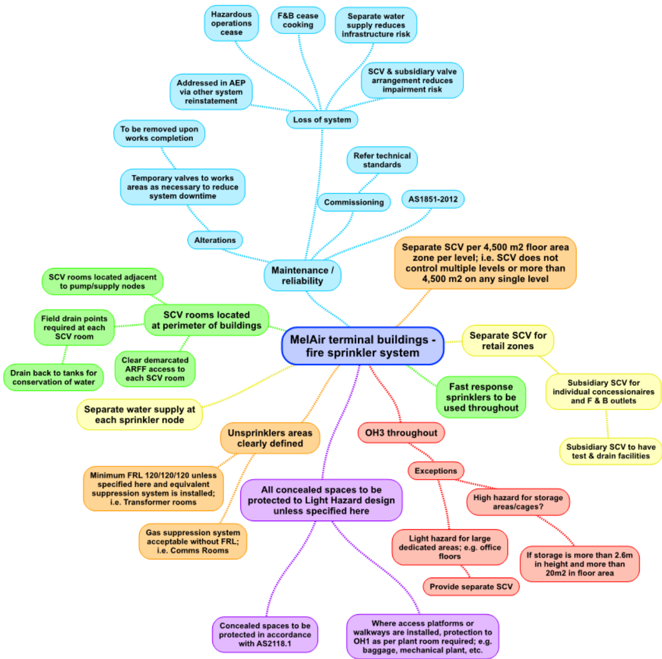
Figure 6.4: Fire Sprinkler System Concept Design Features
