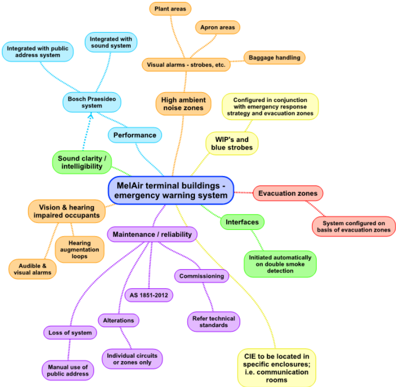
Figure 6.5: Emergency Warning System Concept Design Features
