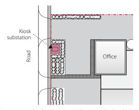
Figure D.3.10 - Locate kiosk substations within site setbacks where possible  $\,$
