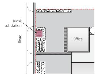
Figure D.2.8 - Locate kiosk substations within site setbacks where possible
