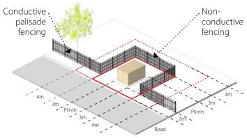
Figure D.4.9 - An acceptable approach to screening a Kiosk Substation
