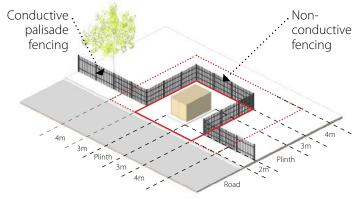
Figure D.2.7 - An acceptable approach to screening a Kiosk Substation
