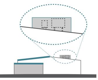
Figure D.1.4 - Roof forms for entry and office areas should be distinct from industrial parts of the building and appropriately screened.
