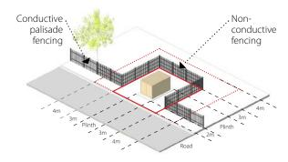
Figure D.3.9 - An acceptable approach to screening a Kiosk Substation
