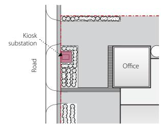
Figure D.4.8 - Locate kiosk substations within site setbacks where possible
