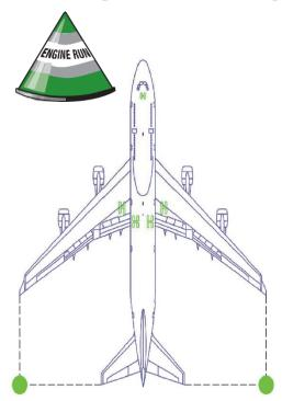
Green engine run cones indicate when an engine ground run is underway. The cones are green with a reflective stripe.
