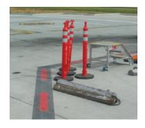
Equipment Staging Areas are defined by a broken red line and are set aside for the staging of equipment and vehicles, prior to an aircraft arrival, while it is on the bay & for a short time after its departure (up to 15-20 minutes).
