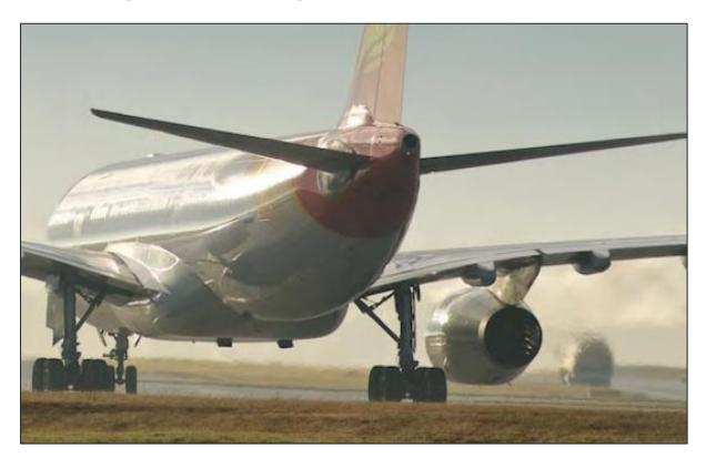
Jet Blast is the exhaust emission from a jet engine. It will be hot, contain noxious gasses, travel at high speeds and can blow loose material around. Always stay at least 75 metres away from the rear of an operating engine to avoid jet blast.
