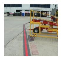
Equipment Storage Areas are defined by a solid red line and are set aside for the parking of airline equipment and vehicles in the medium term (up to 24 hours).
