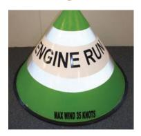
A cone of the same size and shape as the more common unserviceability cone. Indicates an engine ground run is underway.
