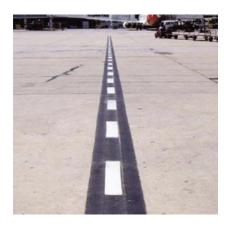
Aircraft are pushed back along a broken white line. The line provides an indication of the path for the tug to follow.
