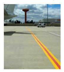
A solid red line bordered by yellow lines, confirming clearance to both parked and taxiing aircraft. When driving past parked aircraft stay to the taxilane side of this line. If aircraft are using the taxilane, stay on the bay side of the line, while remaining clear of parked aircraft.
