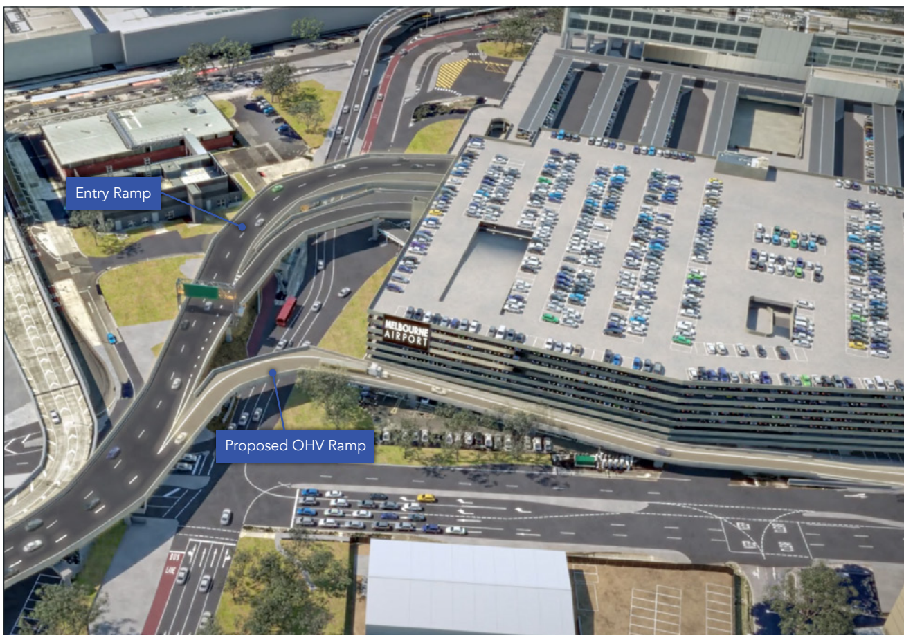
Figure 2: Proposed variation to the Elevated Road and Forecourt Project Stage 2 design, with the OHV ramp location moved for vehicles to exit onto Centre Road
