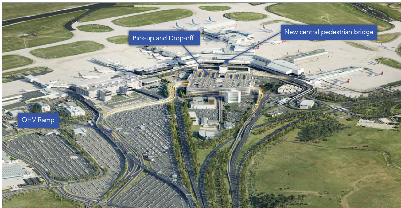
Figure 1: Elevated Road and Forecourt Project Stage 2 design, with the initial over height vehicle (OHV) ramp that moves vehicles onto Airport Drive
