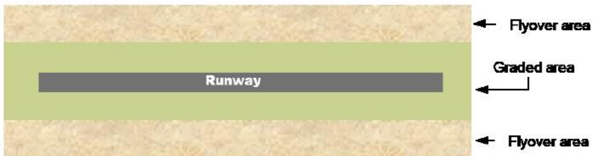
Figure 1: Composition of a runway strip
